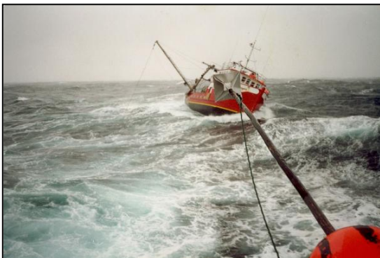
Figure 5.0 (c)(i): Fishing vessel takes a severe roll due to adverse broadside sea conditions. (Source: unknown)
