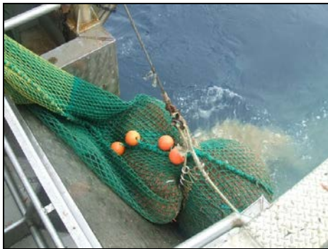
Figure 5.0 (a)(v): Lifting aboard large weights in the cod end as well as the temporary storage of catch on deck, or in an hopper above the deck, negatively impacts the vessels stability. (Courtesy of J.G. personal collection)
