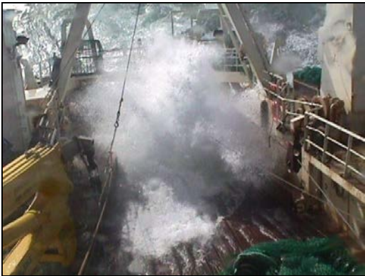
Figure 5.0 (a)(viii) Large fishing vessel with its trawl fast upon an obstruction, stern to the sea conditions
