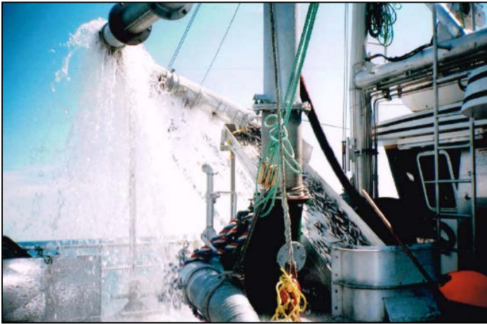
Figure 7.0 (b)(i): Fish being pumped on board, passing through the dewatering system on board the F/V 'Newfoundland Spirit'. (Courtesy of J.G. personal collection.)
