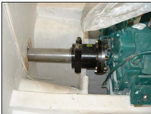
Figure 3.0 (a)(i); Bulkhead replaced after transmission was replaced in a small fishing vessel. (Source: unknown)
