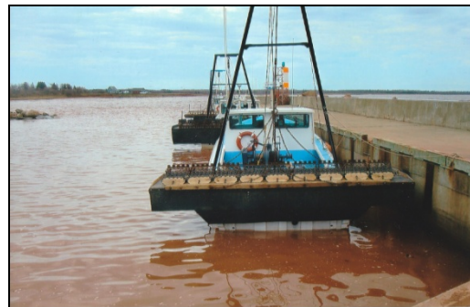
Figure 5.0 (a)(v): Lifting aboard large weights in the cod end as well as the temporary storage of catch on deck, or in an hopper above the deck, negatively impacts the vessels stability. (Courtesy of J.G. personal collection)
