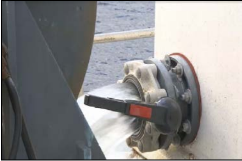
Figure 4.0 (g)(ii): Anti-roll tank dump valve, on board of a fishing vessel. (Courtesy of FVSS – CCPFH)
