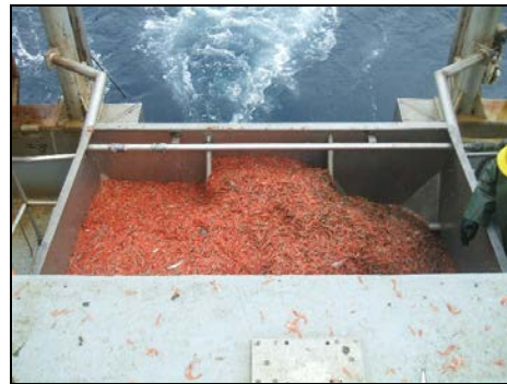
Figure 5.0 (a)(v): Lifting aboard large weights in the cod end as well as the temporary storage of catch on deck, or in an hopper above the deck, negatively impacts the vessels stability. (Courtesy of J.G. personal collection)
