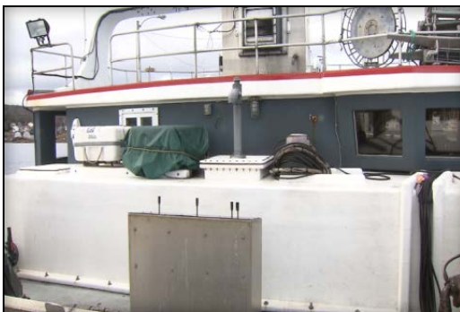
Figure 4.0 (g)(i): Typical anti-roll tank installed on board of a fishing vessel. (Courtesy of FVSS - CCPFH)
